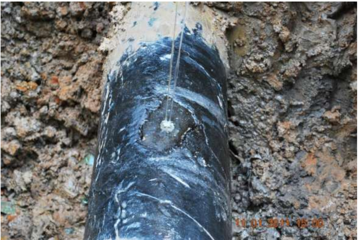
Close-up: Leak from a hole on 10" Kokori Pipeline . Picture was taken during JIV of 11 January 2011
