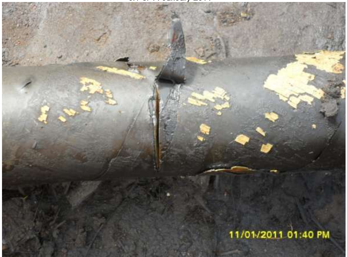
Close-up: Cut on Ubie Well 9S Flowline . Picture was taken during JIV of 11 January 2011
